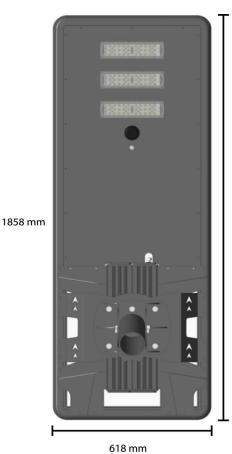
1638 mm 60W Packing Dimensions 1 solar light per box 1645L X 635W X 160H mm
